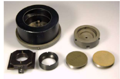
Fig. 2: Specimen holder for ring/area for hydraulic oils and gear oils with coated specimens
